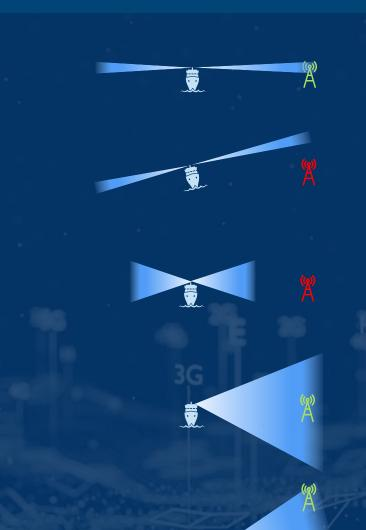
9dB omni 12° angle Can reach the Node Unstable when > 6° inclination
